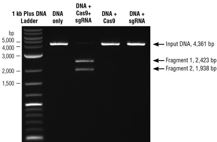
DNA target is *PvuII*-linearized *pBR322*, sgRNA was synthesized using the EnGen sgRNA Control Oligo, *S. pyogenes*. Reactions were set up following NEB® protocols with a ratio of 20:20:1 (Cas9:sgRNA:target site) in 30 µl reactions. Aliquots of reactions were mixed with Gel Loading Dye, Purple (6X) (NEB #B7024). Cleavage products and 1 kb Plus DNA Ladder (NEB #N3200) were resolved on a 1% TBE agarose gel stained with ethidium bromide.
