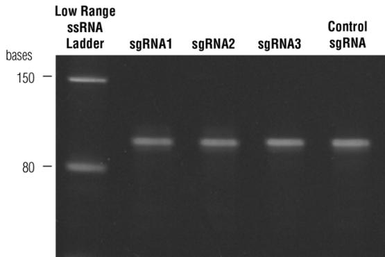
RNA was run under denaturing conditions on a 10% Novex TBE-Urea gel and post-stained with SYBR Gold.
