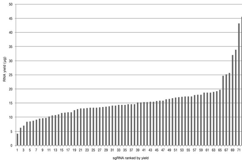
72 different target-specific oligos were designed and tested for RNA yield following DNase I treatment and column purification as determined by NanoDrop. RNA yields may be dependent on specific oligo sequence, with most falling between 4–25 µg.
